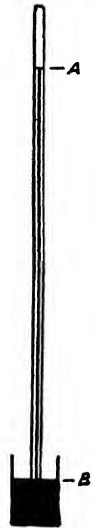
FIG. 30.—Diagram showing a mercury barometer. The tube is filled with mercury and is inverted over a cup with mercury. The mercury column falls until AB balances the pressure of the air at the place where the barometer is located.
